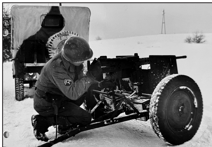
This homemade field piece, especially designed for street fighting, was built by T/5 Dale P. Curtis, Co. F, 2nd Bn, 379th Reg., 95th ID of Granville, Ohio. Using scrap pieces, he reconverted a .50 cal. machine gun and equipped it with a 20 power scope. The gun was used for street fighting in Saarlautern, Germany, and was commended by all who saw it in action. Wallerfangen, Germany, 1/26/1945.
